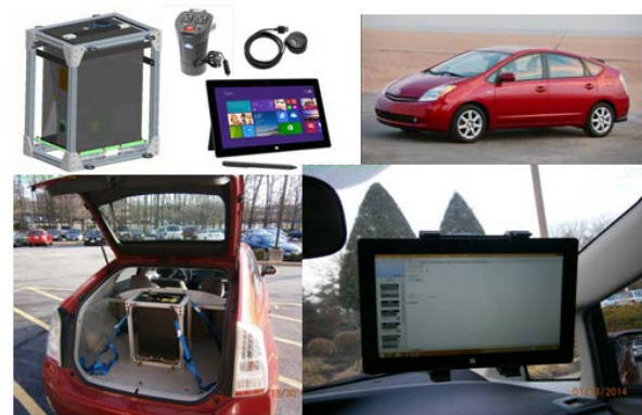
Figure 1. The mobile lidar kit consists of a MiniMPL, a car mount, power inverter, GPS and Microsoft Surface Pro tablet.
